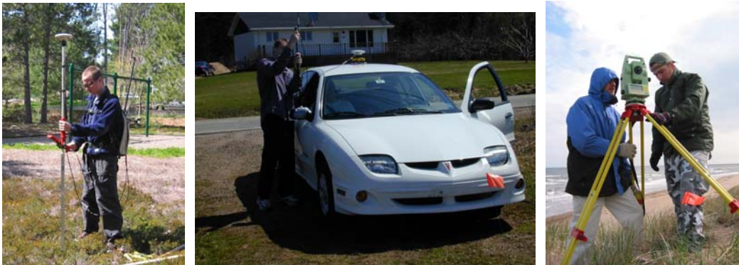
Figure 8 – GPS data were collected with a Leica RTK system on a pole (left), on top of a vehicle (middle), and with a total station unit (right).
