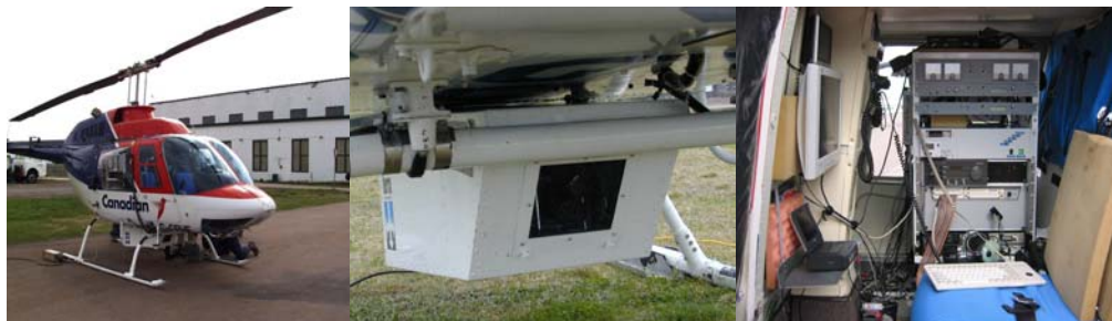
Figure 3 – Terra Remote Sensing LIDAR setup showing the aircraft (left), the sensor mount (middle) and the equipment inside of the aircraft (right).
