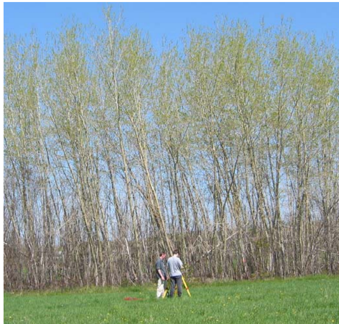
Figure 22 – Setting up the Total Station unit outside of a forest stand.
